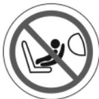
\* Backward facing child restraint systems may never be used with an activated front airbag!
